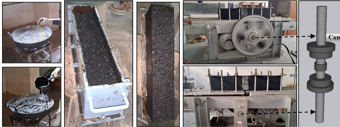
Fig. 8. Beam casting and reflection crack simulator setup
