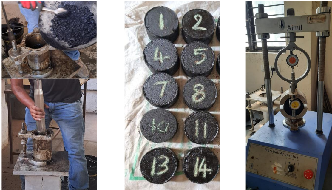
Fig. 6. Casting and testing of marshall specimens
