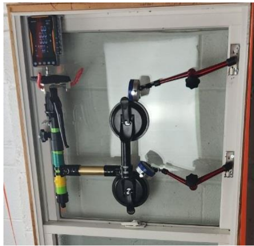
Fig. 3. Mounting device for point loading of double-glazed windows
