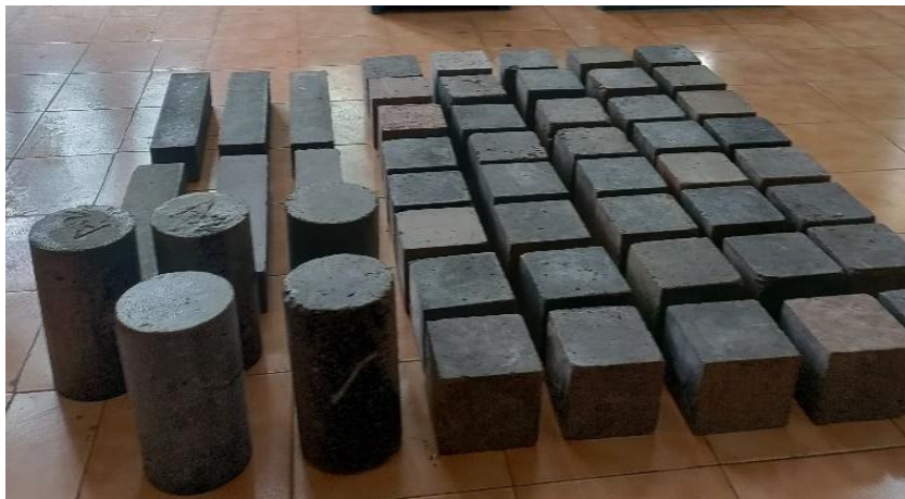
Fig. 2. Concrete samples prepared for strength testing
