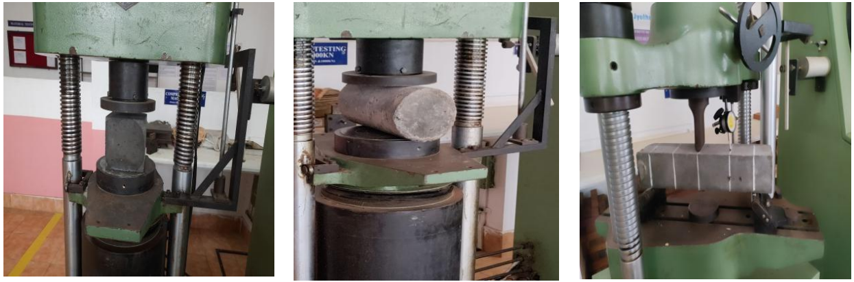
Fig. 4. Experimental setup for Mechanical strength testing
