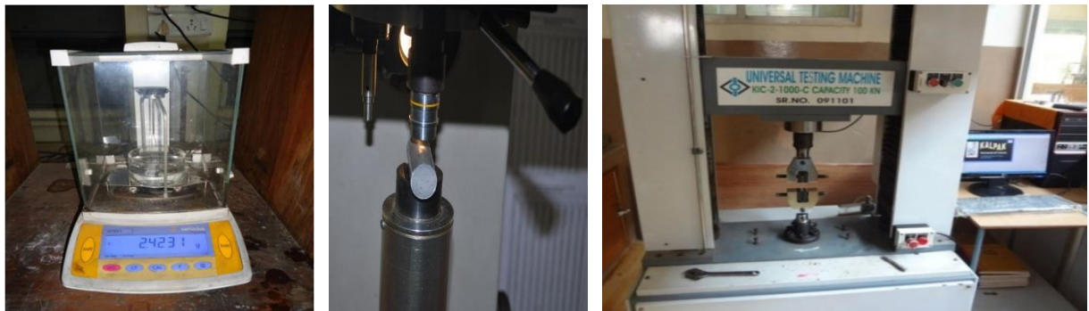
Fig. 4. Density tester, hardness test setup, UTM for tensile properties
