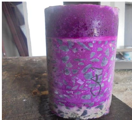
Fig. 10. Carbonation for Phase 1 Mix (0% RAC-Control-CA1) concrete sample
