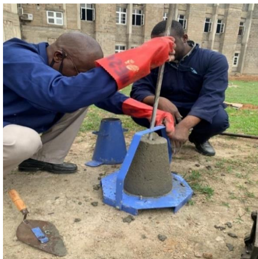
Fig. 7. Experiment on the workability of concrete specimen
