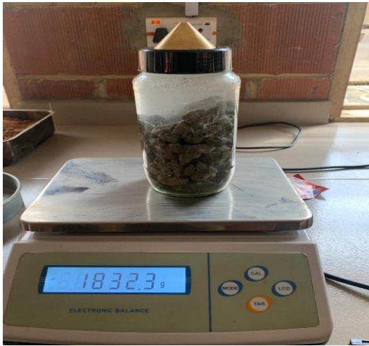
Fig. 3. Particle Density Apparatus – Pycnometer Technique
