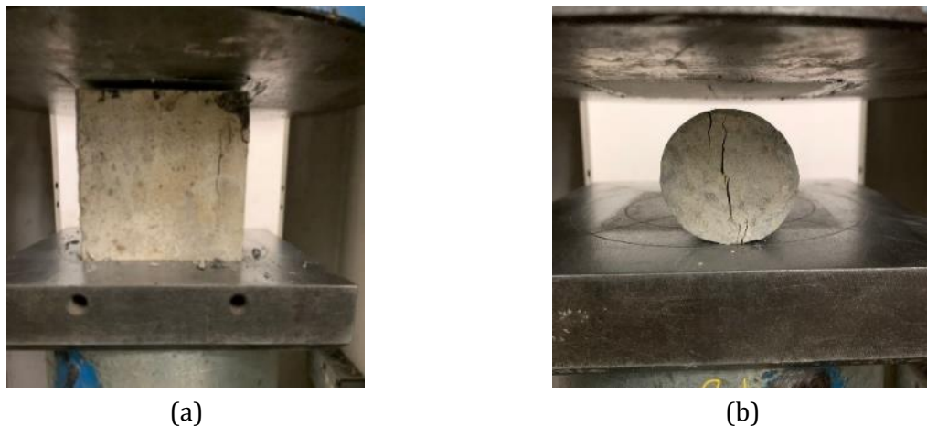
Fig. 10. Experimental setup of HFC specimens under compressive loading and split tensile strength: (a) cubic specimen; (b) cylindrical specimen
