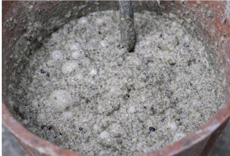
Fig. 1. Fresh polyurethane foam concrete mix during laboratory mixing, showing uniform foam dispersion within the cementitious matrix
