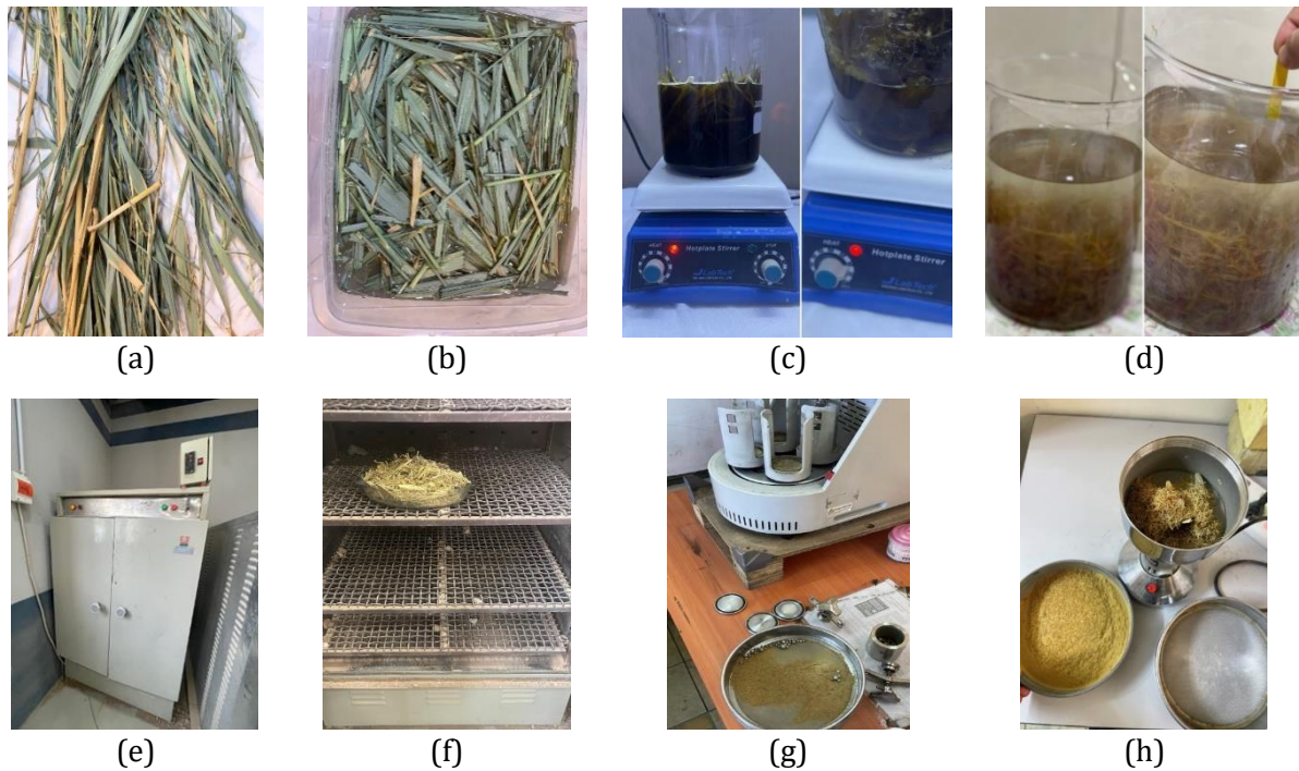
Fig. 1. (a) Materials (b) Cutting & Washing. (c) alkali treatment by 4% NaOH. (d) Washing with distilled water (neutralization). (e), (f) Drying Process. (g) Blender process (h) Milling Process
