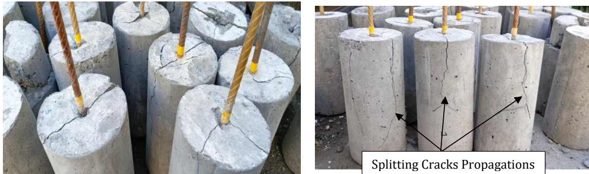
Fig. 6. failure modes of the examined specimens
