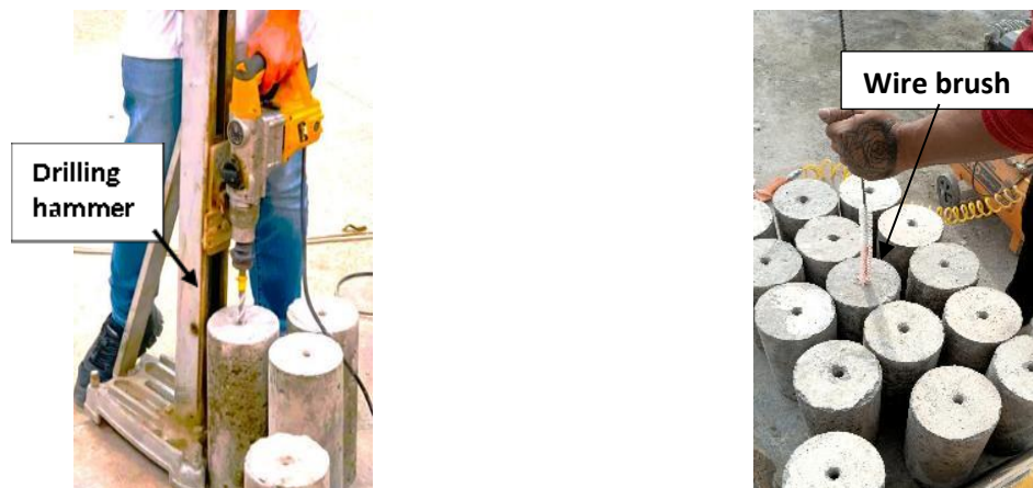
Fig. 2. Drilling and cleaning of the holes
