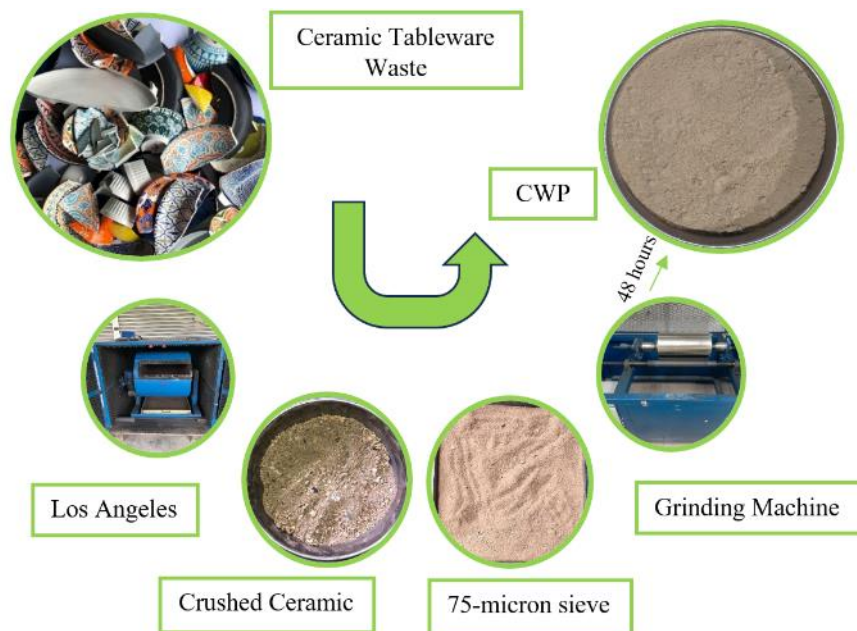
Fig. 1. Preparation procedure of CWP from discarded ceramic materials
