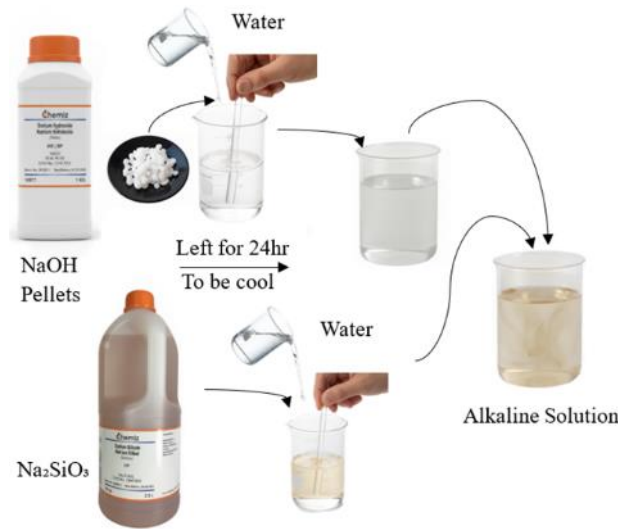
Fig. 4. Procedure for the alkaline activator solution preparation
