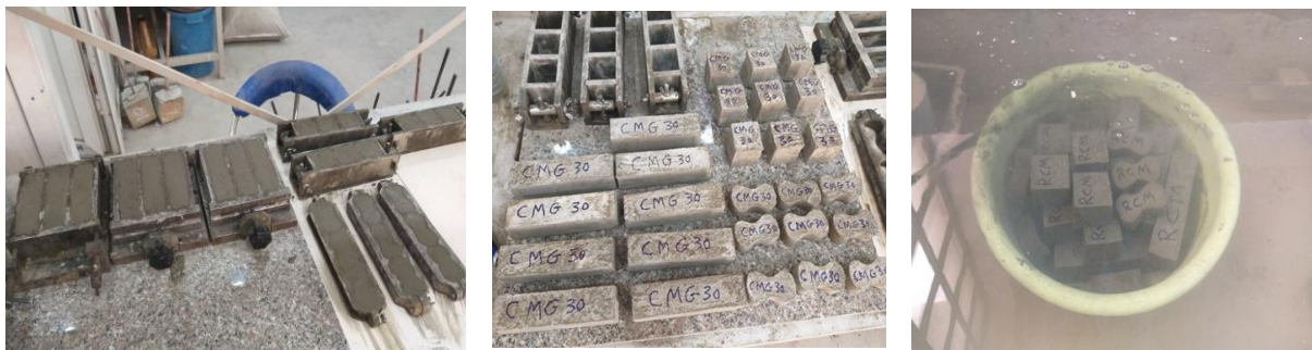
Fig. 2. Casting, remolding, and curing of specimens
