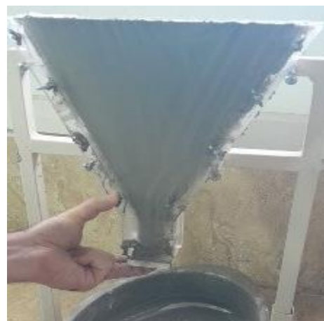
Fig. 3. Flow time test using the V-funnel
