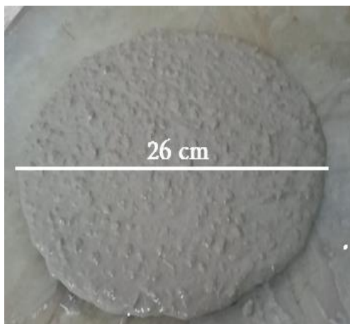
Fig. 2. Slump flow test using the mini-cone
