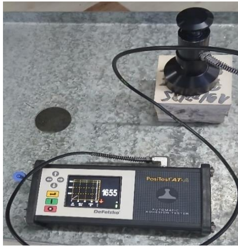
Fig. 5. Apparatus used to evaluate the bond strength between the concrete substrate and the SCSC repair layer
