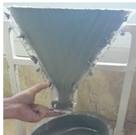
Fig. 3. Flow time test using the V-funnel
