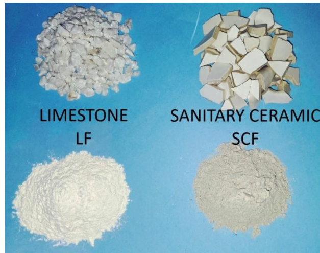
Fig. 1. Limestone fillers (LF) and sanitary ceramic fillers (SCF) in their raw and ground states
