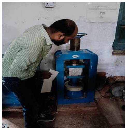
Fig. 1. Compressive strength testing machine
