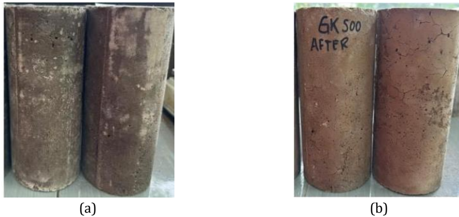
Fig. 10. The figures show the physical condition of geopolymer concrete specimens prior to and after exposure to 500°C: (a) before burning, dark gray in color; (b) after burning, showing a slight orange hue, fine cracking, and no evidence of spalling
