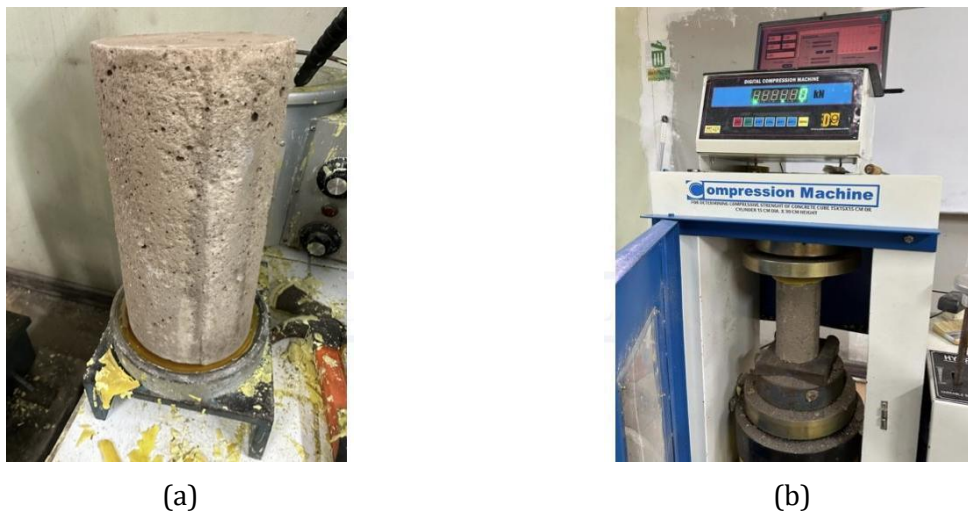
Fig. 6. Compressive strength test: (a) cured and heated concrete prior to testing and (b) specimens testing using a universal compression testing machine
