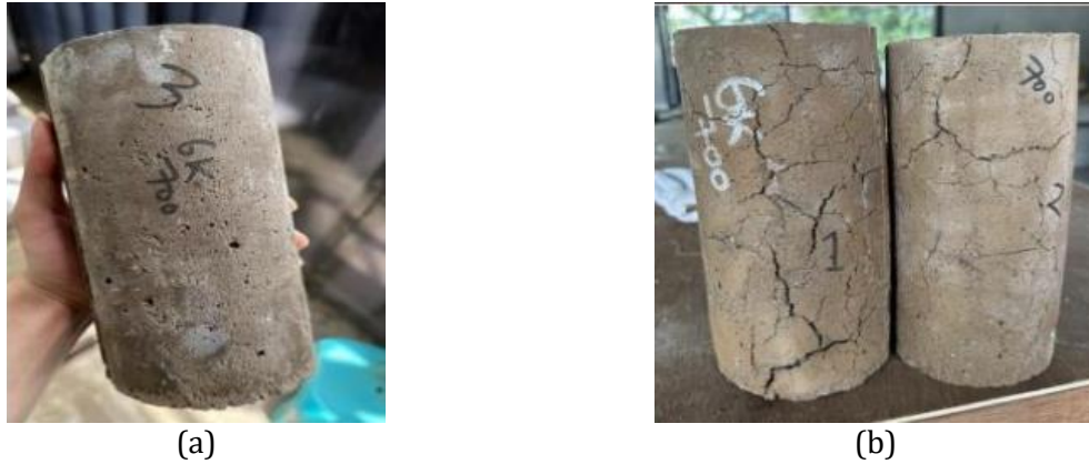
Fig. 14. Physical condition of geopolymer concrete specimens before and after exposure to 700°C: (a) before burning, dark gray in color; (b) after burning, showing a brownish-gray color with reddish accents in some areas, more extensive cracking, no evidence of spalling, and noticeable expansion
