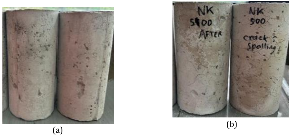
Fig. 9. Physical condition of normal concrete specimens before and after exposure to 500°C: (a) before burning, bright gray in color; (b) after burning, showing no significant color change, with localized yellowish spots, fine cracking, and spalling
