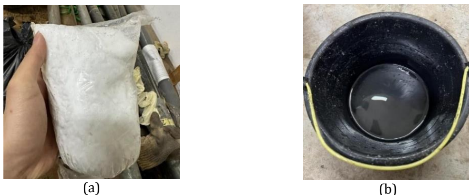
Fig. 1. Alkaline solution consisting of (a) NaOH crystals and (b) NaOH solution
