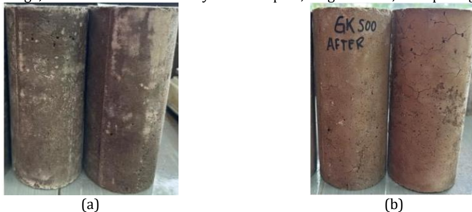
Fig. 12. The figures show the physical condition of geopolymer concrete specimens prior to and after exposure to 600°C: (a) before burning, dark gray in color; (b) after burning, showing a gray-orange color with reddish accents in some areas, more extensive cracking, no evidence of spalling, and noticeable expansion
