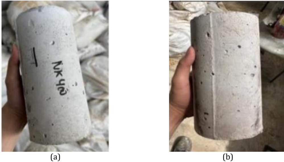
Fig. 7. Physical condition of normal concrete specimens before and after exposure to 400°C: (a) before burning, bright gray in color; (b) after burning, showing no significant color change and fine surface cracks
