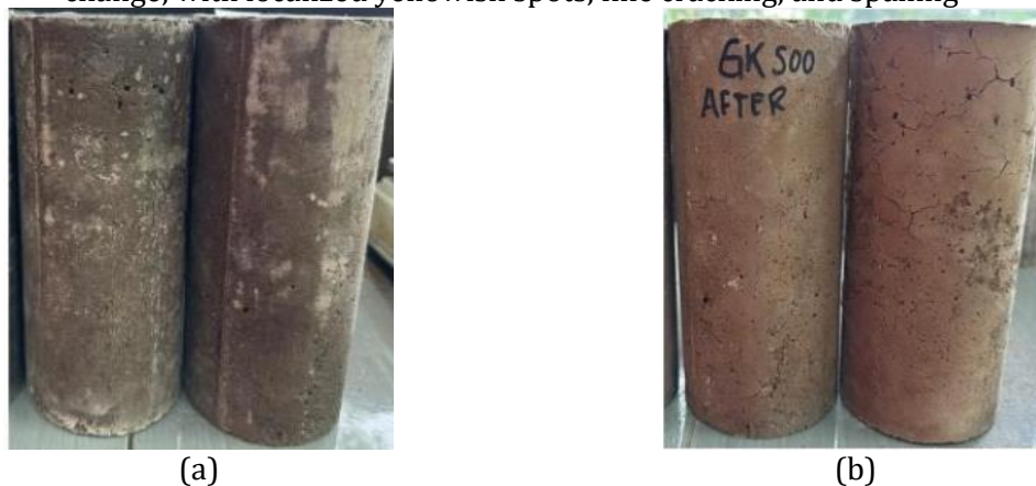
Fig. 10. The figures show the physical condition of geopolymers concrete specimens prior to and after exposure to 500°C: (a) before burning, dark gray in color; (b) after burning, showing a slight orange hue, fine cracking, and no evidence of spalling
