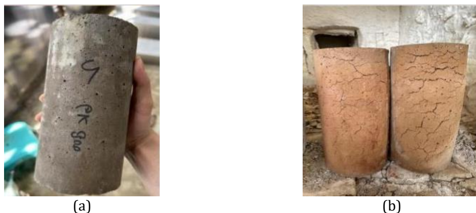
Fig. 16. Physical condition of geopolymer concrete specimens before and after exposure to 800°C: (a) before burning, dark gray in color; (b) after burning, showing a brownish-red color, more extensive cracking, no evidence of spalling, and noticeable expansion
