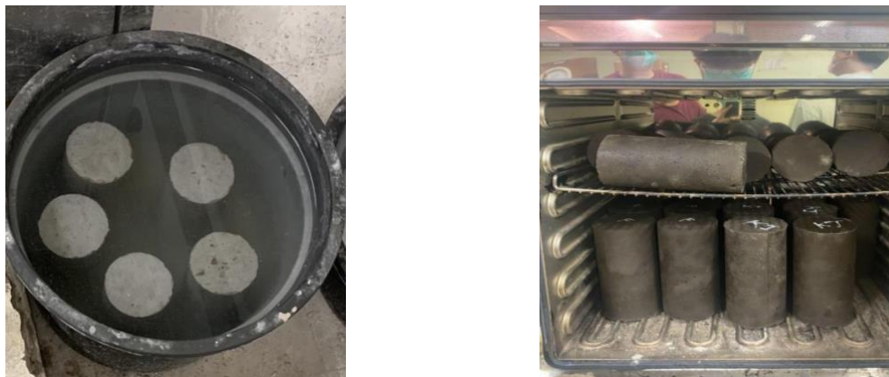
Fig. 4. Curing process of specimens: (a) Submerged curing for normal concrete and (b) heated curing for geopolymer concrete specimens
