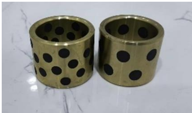
Fig. 1. Bushing from nickel-aluminum bronze with graphite plugs
