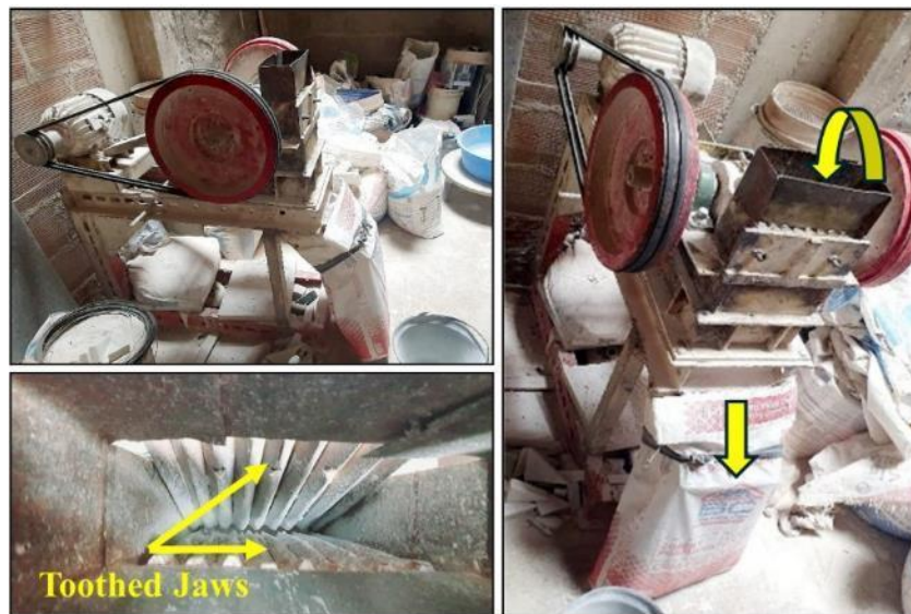
Fig. 1. Toothed jaw crusher used for crushing aggregates
