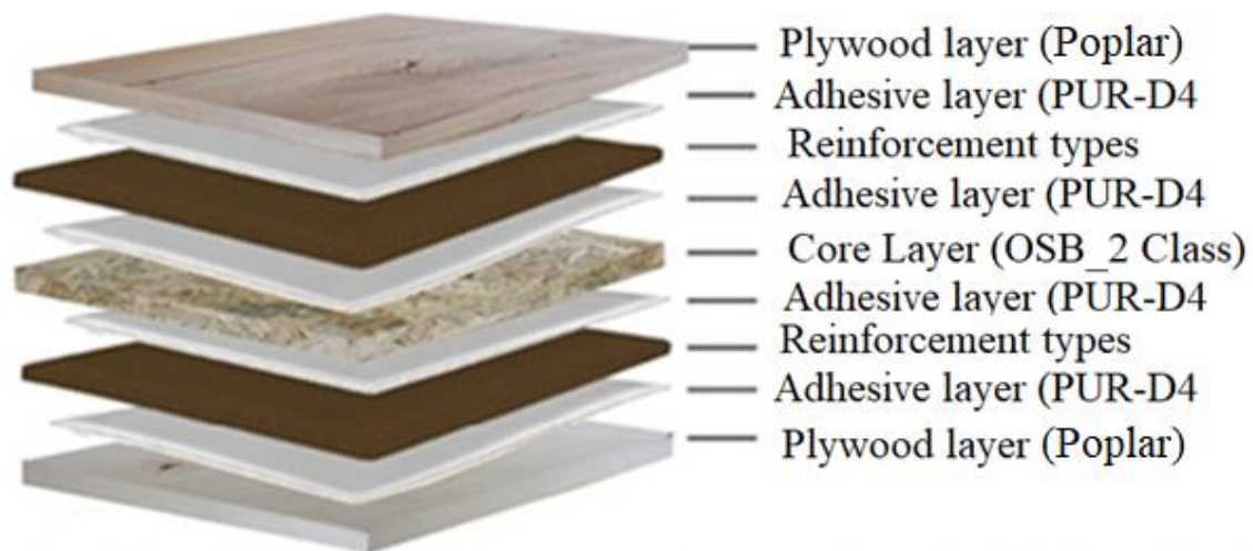
Fig. 3. Exploded view of a multi-layered wood-based sandwich panels structure
