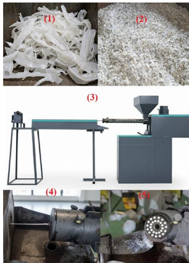
Fig. 4. Stages of recycling polypropylene waste into pellets or 3D-printing filaments
