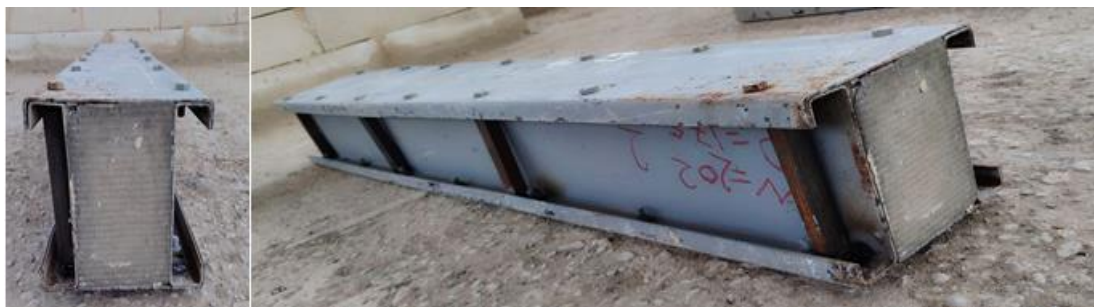
Fig. 21. Failure mode of beam BC1.15
