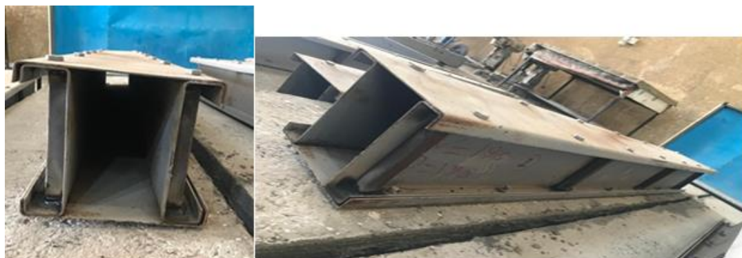
Fig. 11. Failure Mode of Beam BH1
