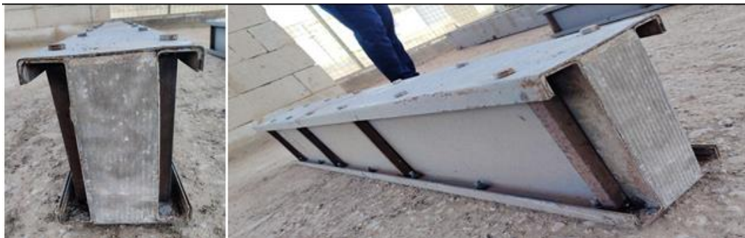
Fig. 24. Failure mode of beam BC0.7
