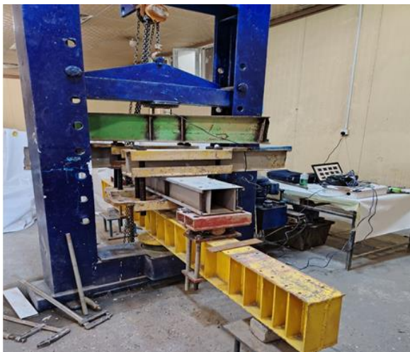
Fig. 6. Member under Torsional load
