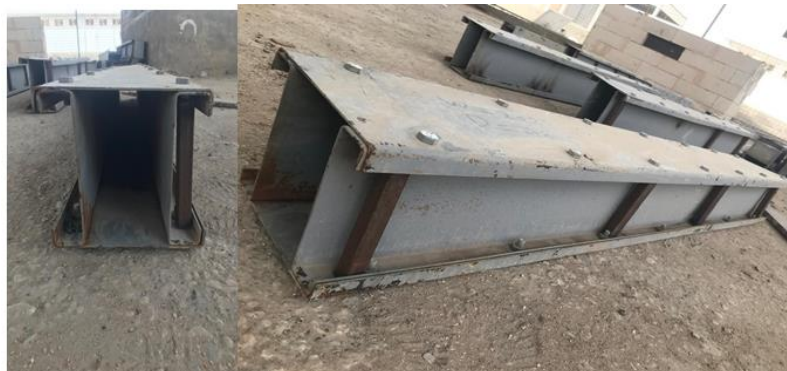
Fig. 9. Failure Mode of Beam BH1.3
