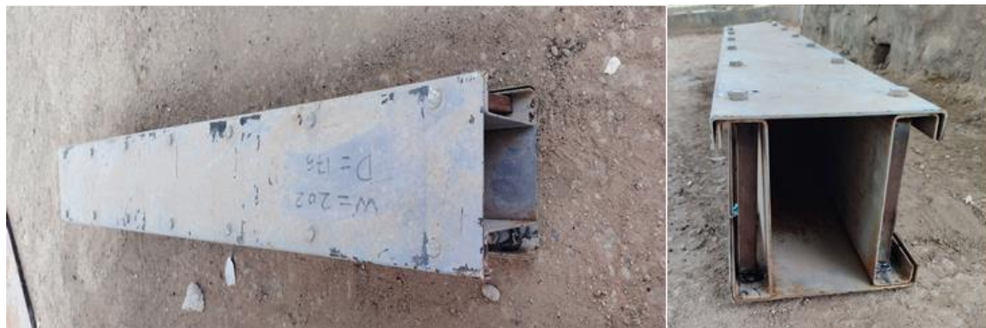
Fig. 10. Failure Mode of Beam BH1.15
