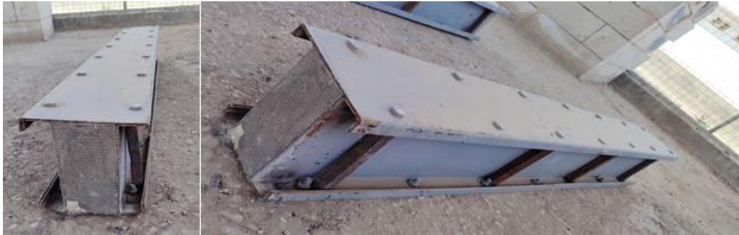
Fig. 23. Failure mode of beam BC0.85
