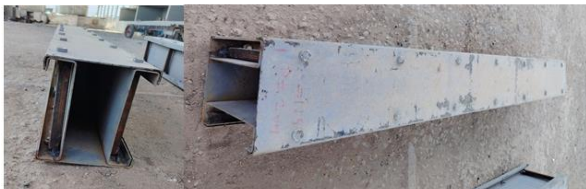
Fig 12. Failure Mode of Beam BH0.85
