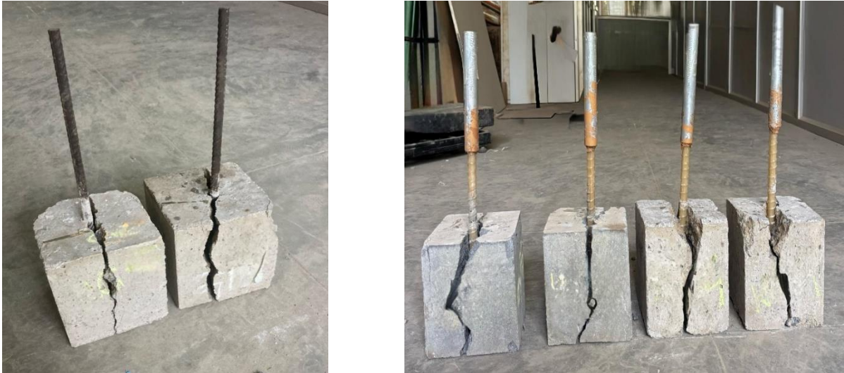
Fig. 4. Failure mode of 12 mm steel bars and GFRP bars in concrete
