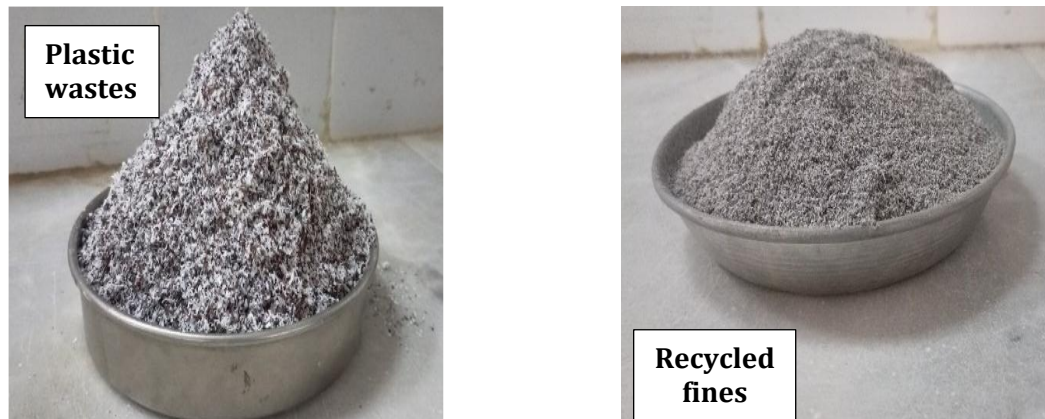
Fig. 2. Recycled fines from plastic waste
