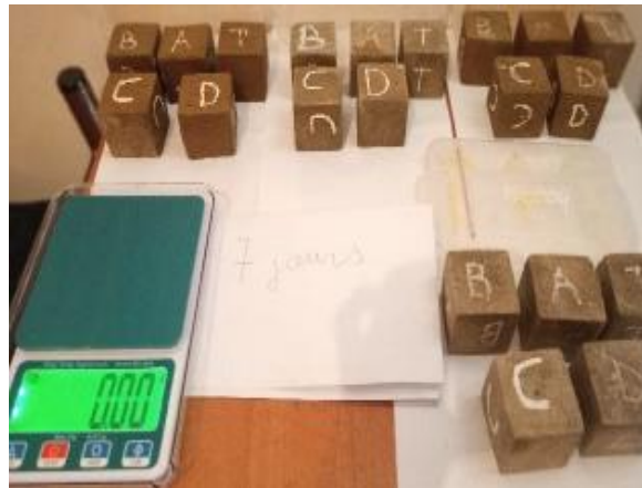
Fig. 14. Measurement of mass loss
