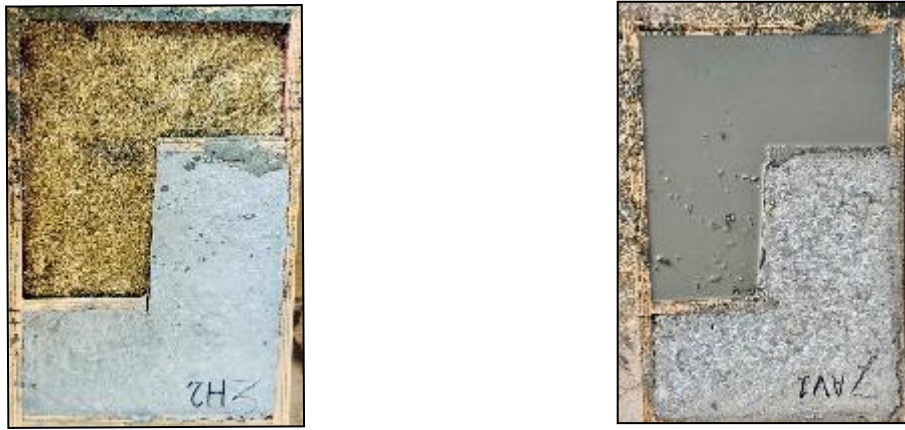
Fig. 4. Casting the second segment of SIFCON concrete
