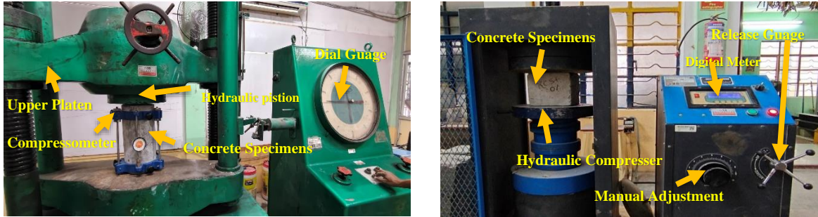
Fig. 3. Experimental test setup of compression testing machine for concrete specimens
