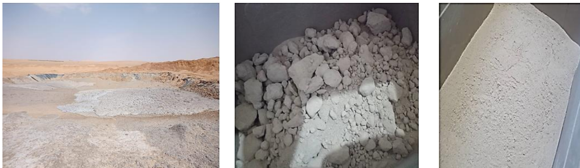
Fig. 2. Treated oil drilling waste before and after grinding
