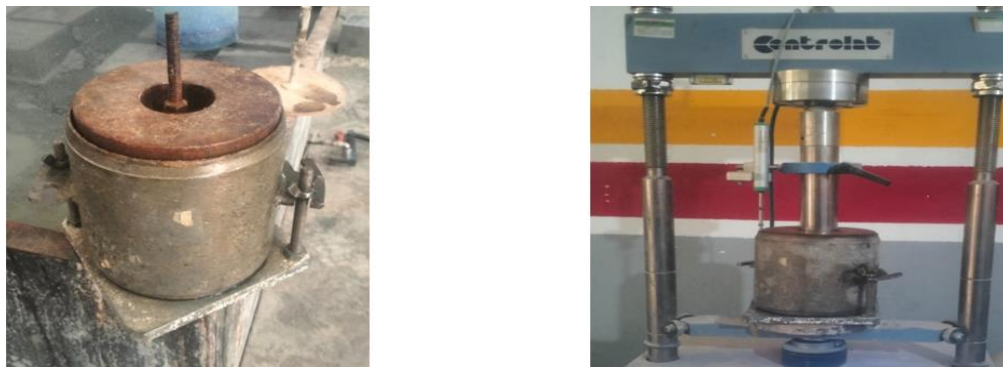
Fig. 4. CBR test for compacted mixtures
