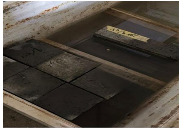
Fig. 4. Curing of specimens
