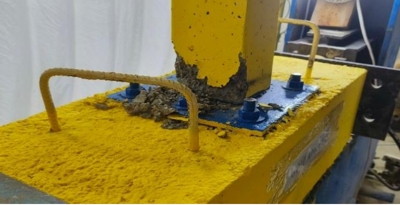
Fig. 24. Failure mode of (6 P10 A16 W1 -5) specimen
