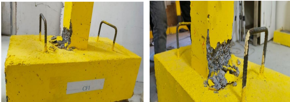
Fig. 19. Failure Mode of CF1 Specimen
