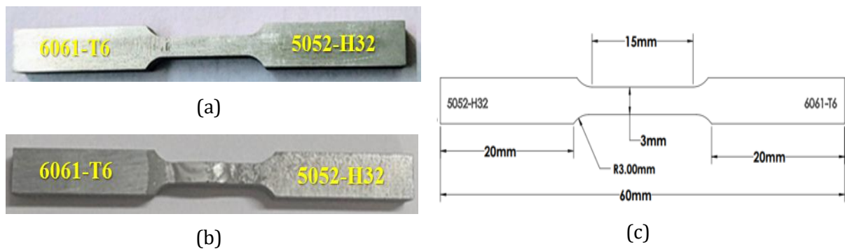
Fig. 4. Extracted micro-tensile specimens: (a) AW specimen (b) PWHT specimen (c) Dimensional schematic
