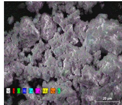
EDS elemental map of PEGP 1% Concrete
