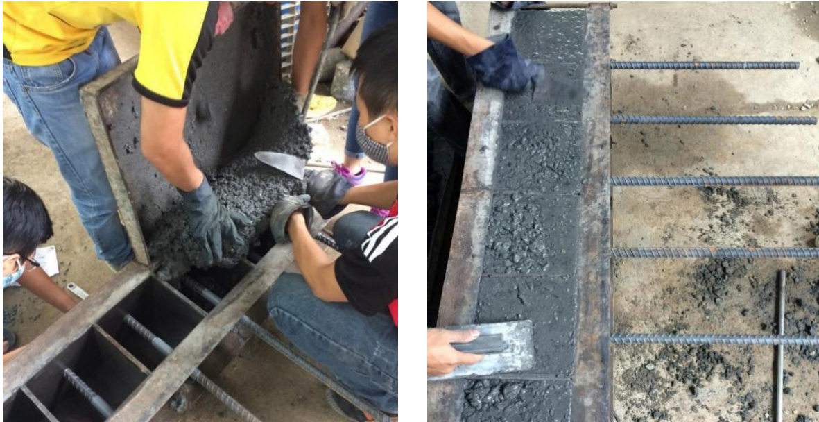
Fig. 2. Schematic of pull-out specimen
