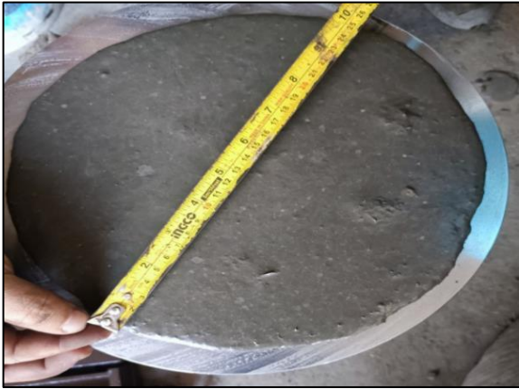
Fig.4. Flow table test of RPC mixtures
