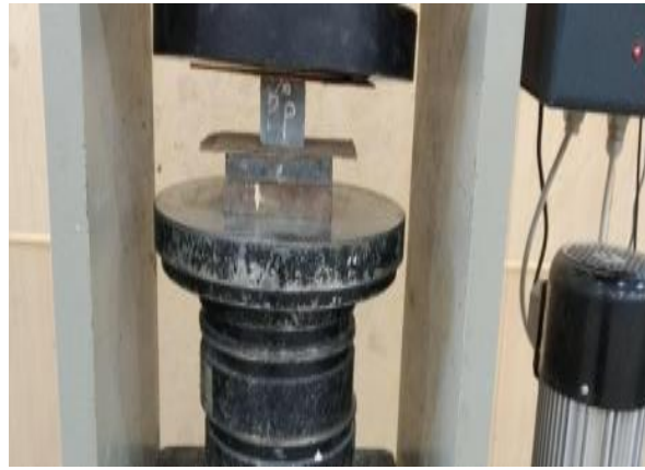
Fig. 5. Compressive strength testing machine used for specimen testing
