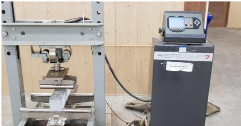
Fig. 6. Flexural strength test setup showing the center point loading configuration for prism specimens
