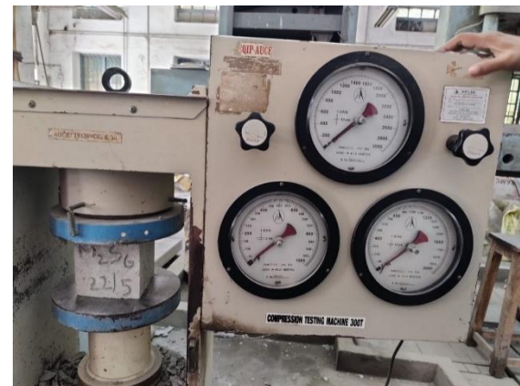
Fig. 5. Experimental setup for compressive strength test
