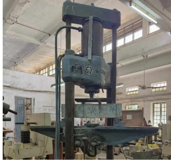
Fig. 7. Test setup for Flexural strength
