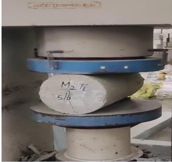
Fig. 6. Test setup for Split tensile strength
