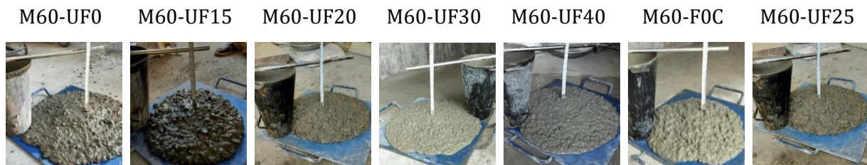
Fig. 7. Slump test conducted on varying UFBFS %, and its influence on workability
