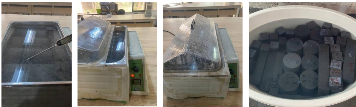
Fig. 3. Hot-water curing of RPC specimens at 70 °C (5 h/day for 3 days), followed by water curing at 20 °C
