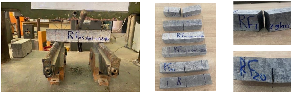
Fig 5. Testing and failure of the specimens
