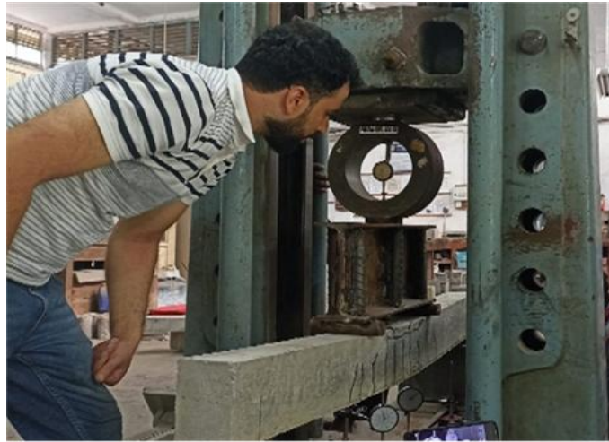
Fig. 4. Flexure strength test setup for four-point bending condition
