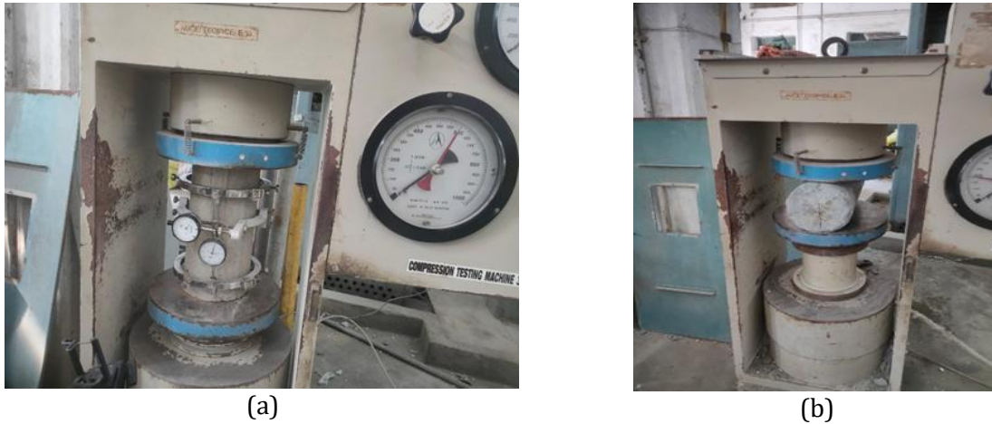
Fig. 3. (a) Uniaxial compressive strength test setup (b) Split tensile strength test setup
