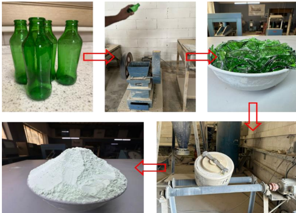
Fig. 2. The process of producing green glass powder less than 45 \mu\text{m}
