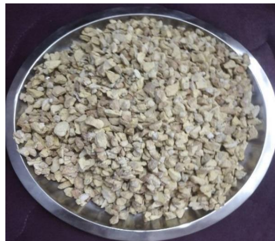
Fig. 7. Attapulgitic lightweight aggregate after PVA treatment, showing the surface coating formed after drying at room temperature for two days
