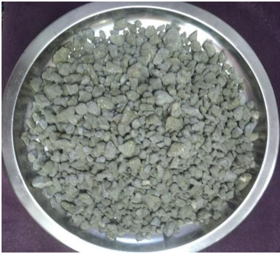
Fig. 4. Attapulgitic lightweight aggregate after cement paste impregnation treatment, showing the formation of a cementitious coating on the aggregate surface prior to curing
