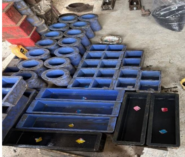
Fig. 8. Steel molds used for casting LWSCC specimens, including cubes, cylinders, and prisms for the different experimental tests
