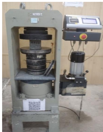
Fig. 11. Compressive strength testing setup
