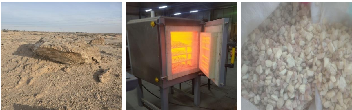
Fig.2. Preparation of attapulgite lightweight aggregate
