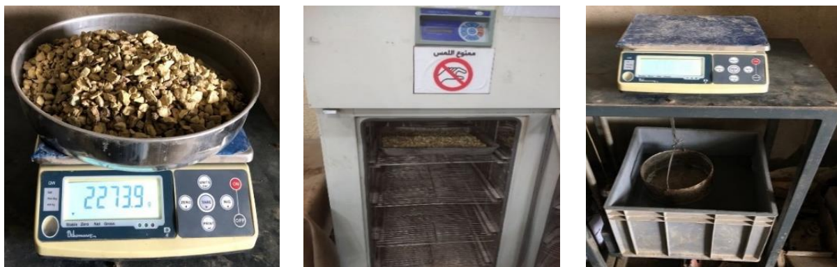
Fig. 9. Main steps of the specific gravity and water absorption test for attapulgite aggregate
