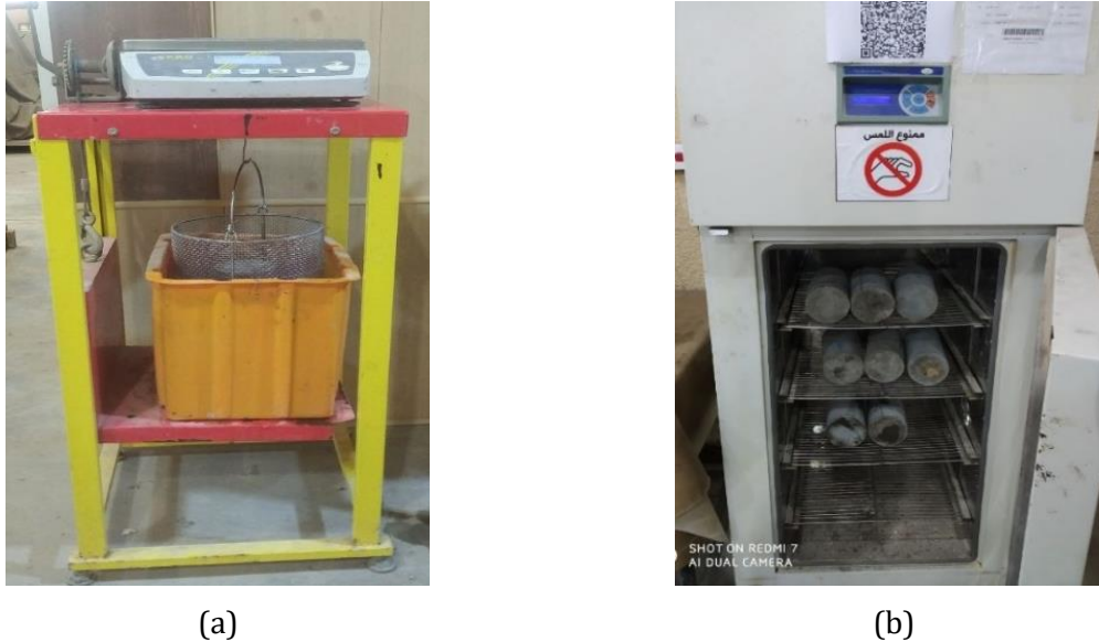
Fig. 12 (a) Apparently submerged mass (A), (b) Oven-dry mass (C)
