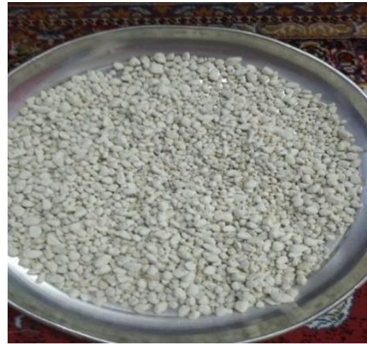
Fig. 5. Attapulgitic lightweight aggregate coated with ceramic adhesive after curing, illustrating the surface sealing effect of the treatment
