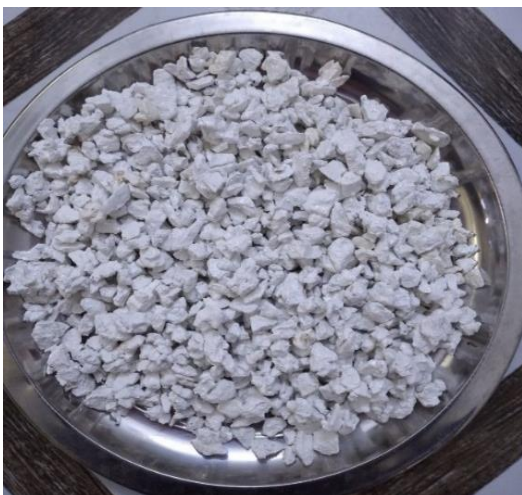
Fig. 6. Attapulgitic lightweight aggregate after gloss enamel paint treatment, showing the formation of a continuous surface coating after two days of drying
