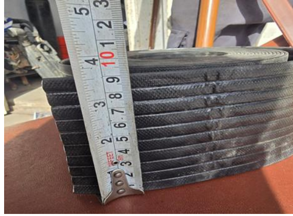
Fig. 2. Paraweb 2D soil reinforcement strips manufactured by Maccaferri
