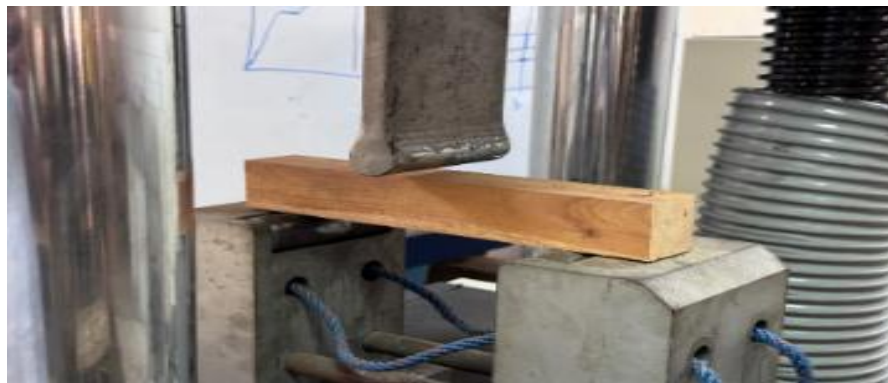
Fig. 1. The three-point bending test according to ASTM D143-22 [4]
