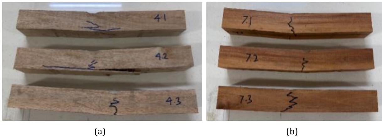
Fig. 3. The three point bending test [4] (a) Red meranti ( Shorea parvifolia ) and (b) Kamper kalimantan ( Dryobalanops lanceolata )
