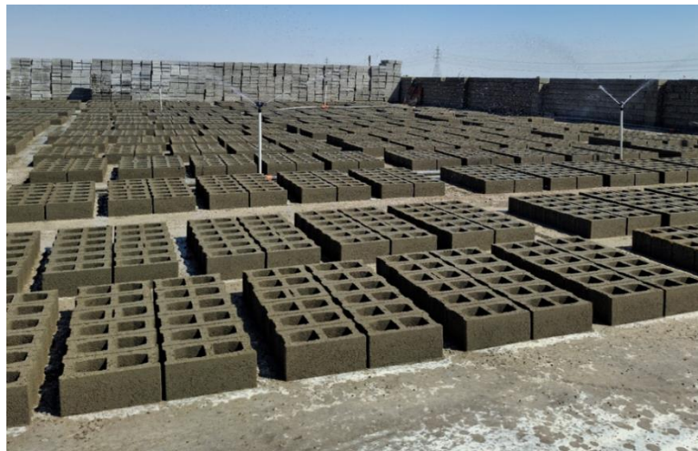
Fig. 8. Curing of manufactured blocks in the plant by water spraying
