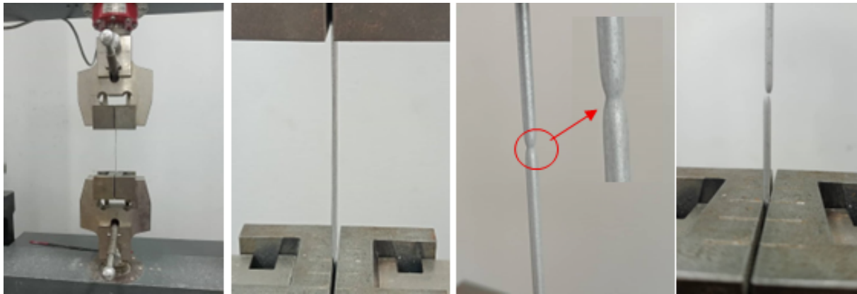
Fig. 3. Galvanized steel tie wire tensile test (necking and fracture)
