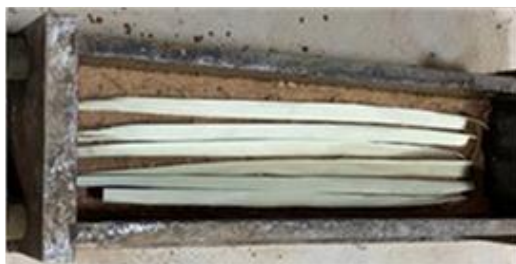
(a) Strips laid on top of a second compacted soil layer
