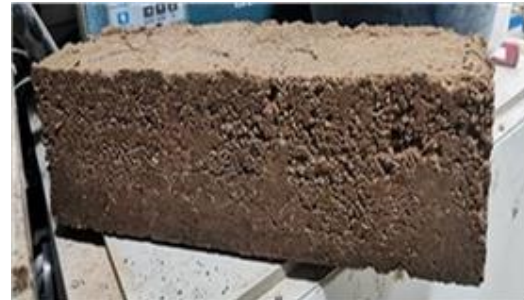
(b) Reinforced soil beam
