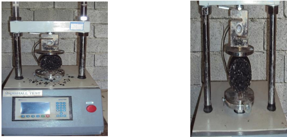
Fig. 3. Illustrative indirect tensile strength test
