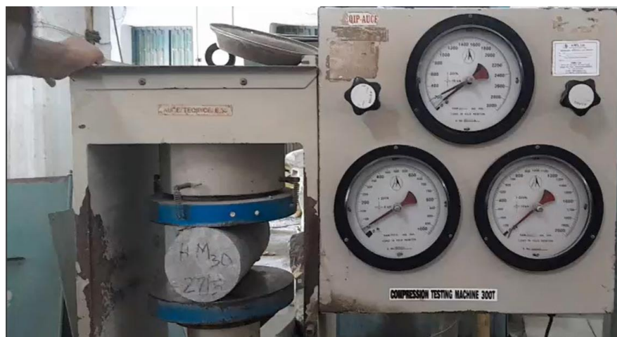
Fig. 3. Split tensile strength testing carried out using a 300T CTM
