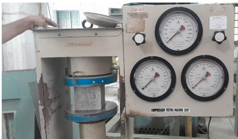
Fig. 2. Compressive strength testing carried out using 300T CTM
