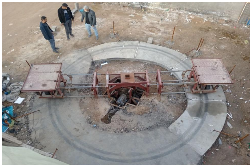
Fig. 1. Photograph of the locally fabricated circular Accelerated Pavement Testing (APT) device
