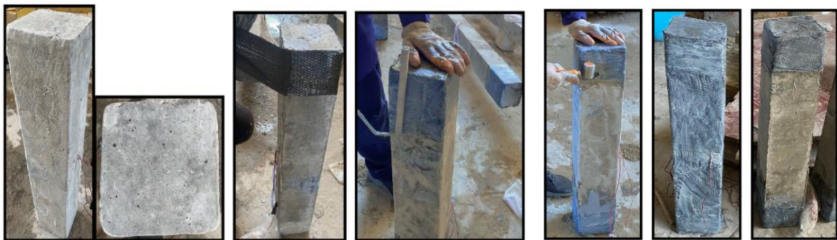
Fig. 5. CFRP strengthening using the wet lay-up technique
