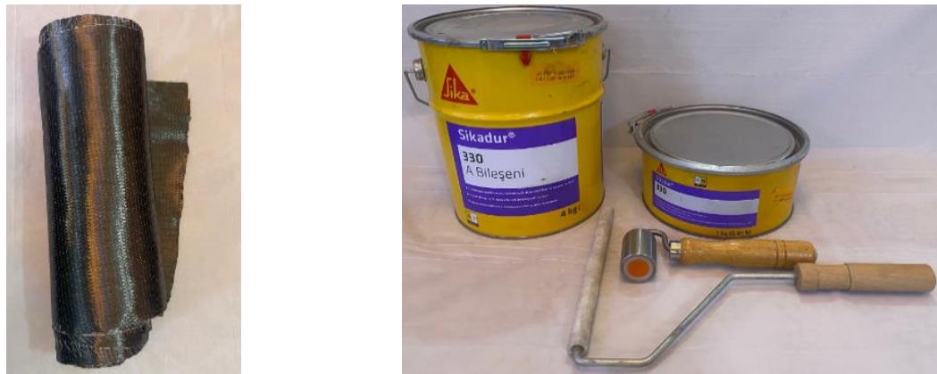
Fig. 2. CFRP strengthening materials and tools: CFRP sheet, epoxy resin, and application rollers
