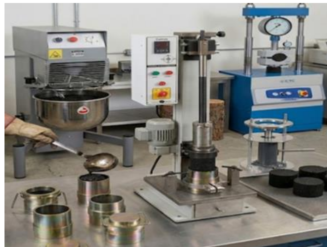
Fig. 2. Marshall testing apparatus and specimen fabrication
