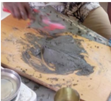
Fig. 2. Cement/CPA paste preparation for determination of physical properties
