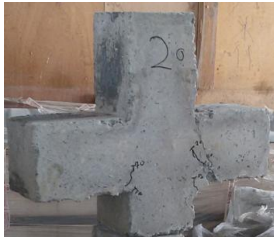
Fig. 14. Crack Pattern of C20 model
