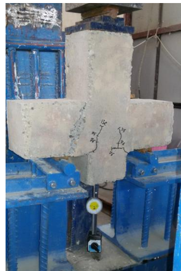
Fig. 10. Specimen within the pressing system during the monotonic test
