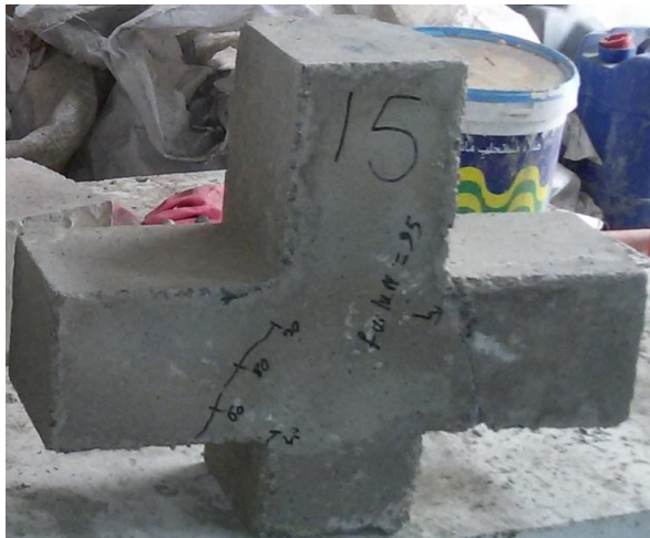
Fig. 13. Crack Pattern for C15 corbel
