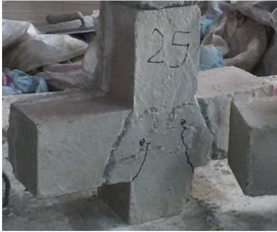
Fig. 15. Model C25 after failure
