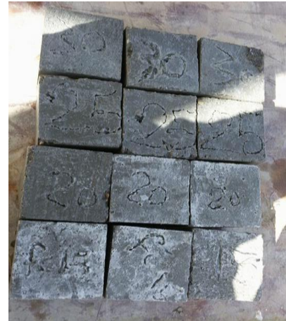
Fig. 8. Corbel specimens and cubes after casting
