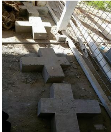
Fig. 8. Corbel specimens and cubes after casting
