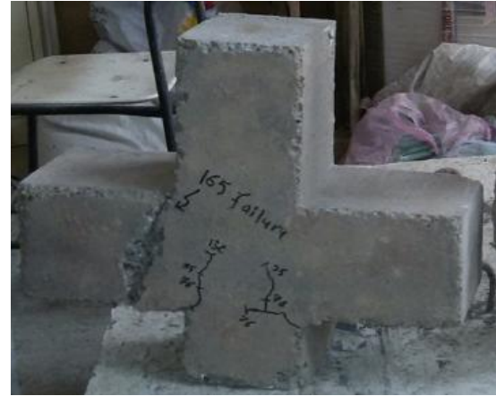
Fig. 16. Crack Pattern of the specimen C30
