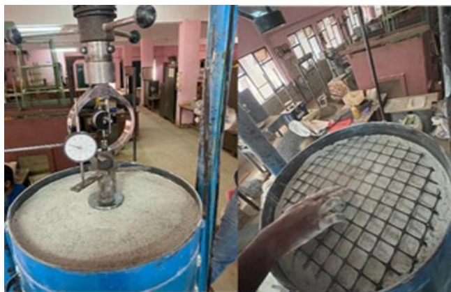
Fig. 4. Preparation of sand bed
